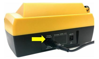
2 Keep the rear of the equipment a minimum distance of 20 cm from any other device or from the wall, so that you do not run the risk of the battery charger plug being pressed or disconnected from the equipment.
